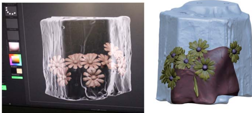
Figure 5. Color-coded digital breakout for molding purposes of a candle with flowers embedded beneath the surface.
