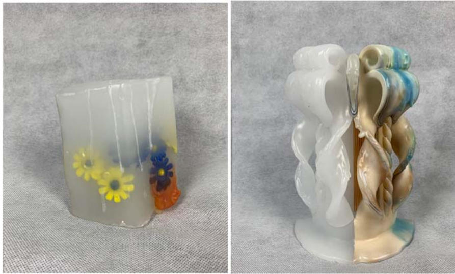
Figure 3. Preliminary samples cast in Smooth On Crystal Clear™ 202. Though very promising, replicated candles displayed deviation of color and transparency that could not be accurately emulated based on the photographic images of the original provided to LifeFormations. Though a fundamentally successful step forward, this exercise proved that completion of the replicated candles side-by-side with the original is essential for successful replication.
