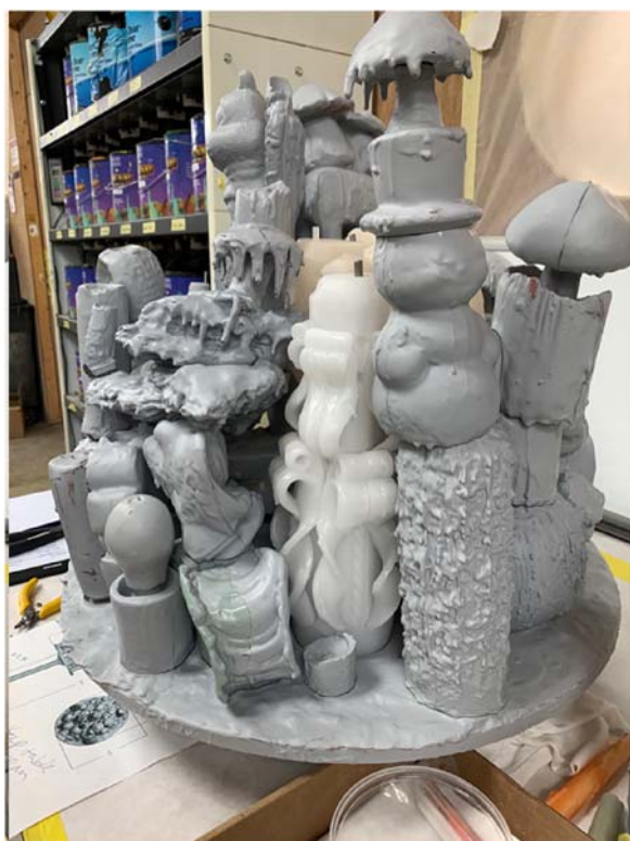
Figure 6. 3D printed candles in Polymer Resin® (gray), hollow casts in Smooth-Cast™ 300 Urethane (white) in a test assembly to define angles and points of registration at LifeFormations' studio.
